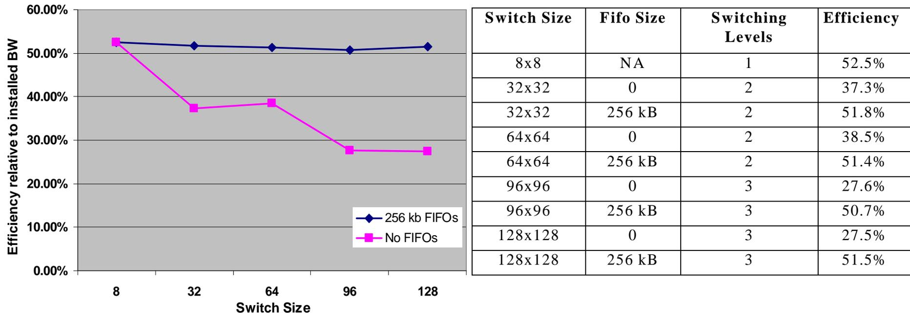
FIFO buffers between switching levels allow to recover scalability
